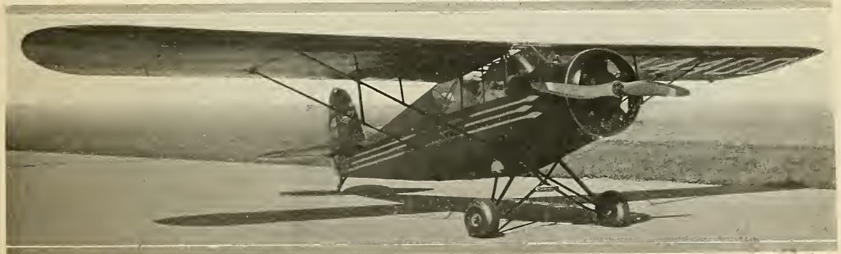
Two-place LeBlond-powered sport plane produced by the Porterfield Aircraft Corp.
